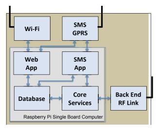
Fig. 1: CATAN System Architecture
