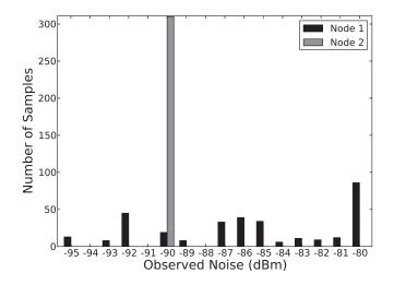
Fig. 4: Observed noise from nodes deployed in field test. (Node 2 was held stationary while node 1 was moving)
