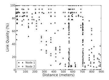
Fig. 5: Relative link quality between nodes 1 and 2 during our field test, as reported by the Ubiquity router.
